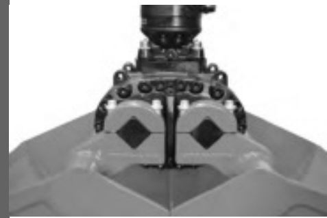
Loosen 4 bolts on each side
