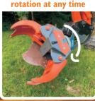
The removable blade on the Echotec TS 300 additionally allows it to be used as a grapple making it multipurpose.
